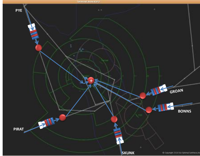
Figure 6. Queuing Network Approximation of the San Francisco Terminal Area Traffic
